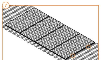
Install all the panels and fasten end clamps at the end of each array.
