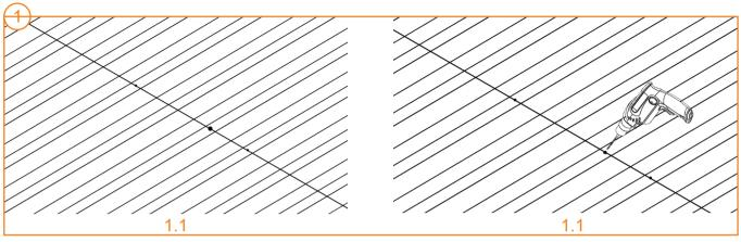
Determine where the roofs mounts will be positioned based on position of existing roof screws, and mark it with a chalk line. Determined a position where the L foot will be attached on a unused crest. Drill a single 6mm pilot hole.
