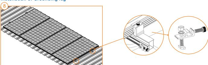
Install a grounding lug onto each rail line edge with an inner hex bolt M8\*25 and a stainless steel nut, then connect 8.4mm² (greater than or equal to 8AWG) copper wire through all the grounding lugs (fixed by M8\*20 inner he x bolt), finally connect a copper wire to the ground. The grounding lug has grounding function when fastened tight to the rail and copper grounding wire.
