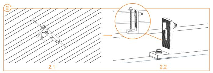
Backfill the pilot hole with sealant then fix the L-foot in place. Fix the L-foot in line.
