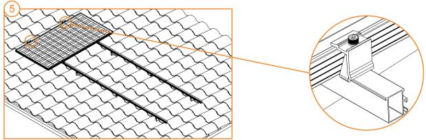
Put the first PV module on the two parallel rails ,fasten the end clamp with inner hex bolts M8 to secure one side of the panel .then slot two mid clamp on the rail.
