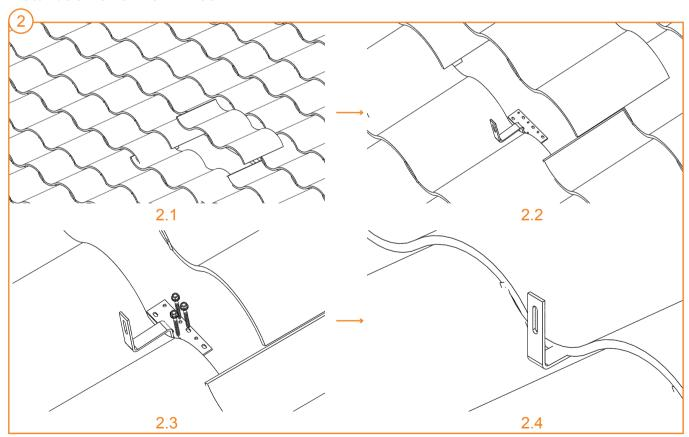
Remove the tile where you are installing the 1# hook by gently pulling and pushing the tile. Place the 1# hook on top of the rafter where it will be installed, then fasten it with three wooden screws M8\*90, finally return the tile to its original position.
