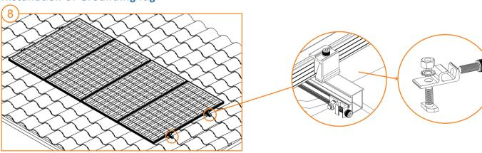
Install a grounding lug onto each rail line edge with an T4 bolt M8\*25 and a stainless steel nut, then connect 8.4mm² (greater than or equal to 8AWG) copper wire through all the grounding lugs (fixed by M8\*20 inner he x bolt), finally connect a copper wire to the ground. The grounding lug has grounding function when fastened tight to the rail and copper grounding wire.
