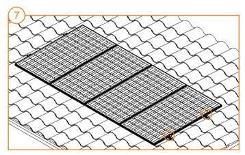
Install all the panels and fasten end clamps at the end of each array.
