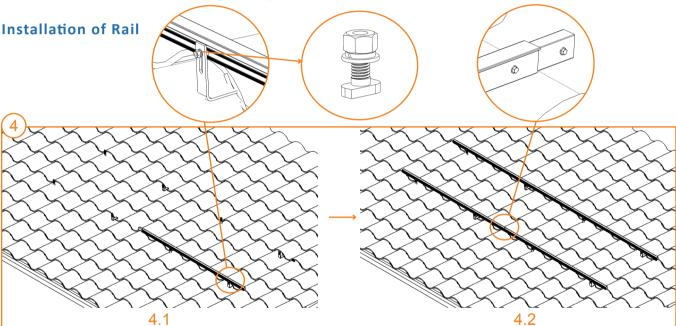
Connect the rail to the 1# hooks with the T-bolt M8\*28 and nut. Fasten to secure. Use the rail splice kit to connect the two rails with the two  $\phi 4.2*12$  self tapping bolts.
