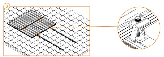
Put the second panel on the rail, fasten the mid clamps with inner hex bolts M8 at all locations where two panels meet .
