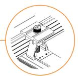
Insert the mid clamp nut by tilting it into the top opening of the rail, then put the second panel onto the rails. Fasten the mid clamps with allen bolts M8 at all locations where two panels meet.
